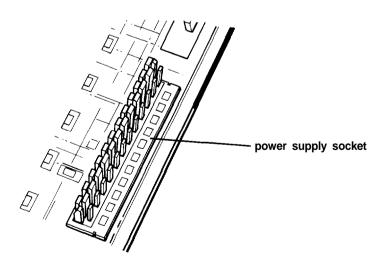
3. Position power supply connector P4 so the large tab on the connector faces the right side of the computer. Beginning with the six pins toward the back of the computer, carefully line up the holes in the connector with the pins in the socket and then push in the connector.
